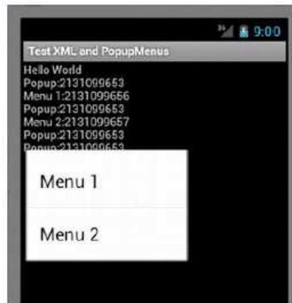
Figure 7–4. Pop-up menu attached to a text view
