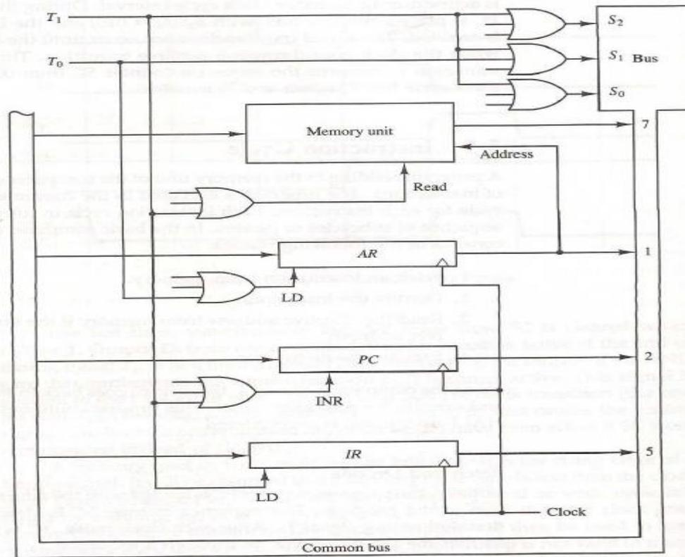
Figure 5-8 Register transfers for the fetch phase.
